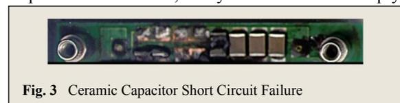
Fig. 3 Ceramic Capacitor Short Circuit Failure
